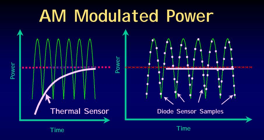
• For diode sensors; power meter accumulates the samples and calculates the average power
