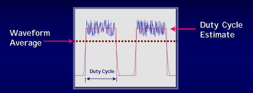
Thermal and average-only diode sensors include measurement errors due to uncertainty of duty cycle, non-ideal pulse, and complex modulation
