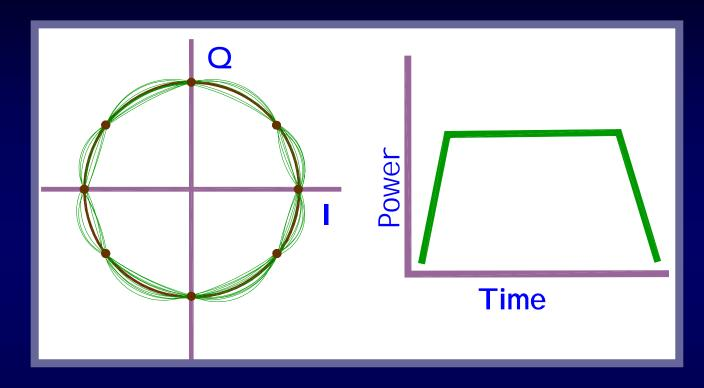
• GSM uses Gaussian Minimum Shift Keying (GMSK) modulation technique
