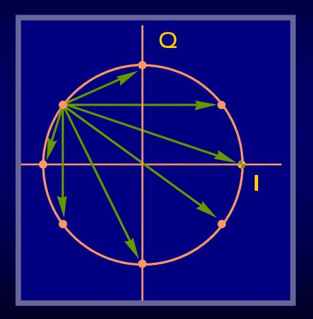
QPSK used in TDMA and CDMA systems Carrier signal is coded using QPSK techniques within the four quadrants at eight positions Transitions from one position to another results in change in amplitude
