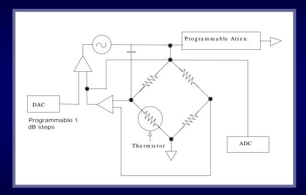
Thermistor used in a patented swept power bridge circuit provides NIST-traceable 90 dB dynamic range
