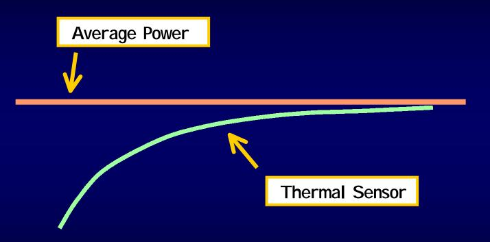
• Thermal Sensors rise to the level of the average power through integration
