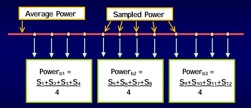
• Diode Sensors sample the average power of a CW signal and store the samples into buckets for further averaging
