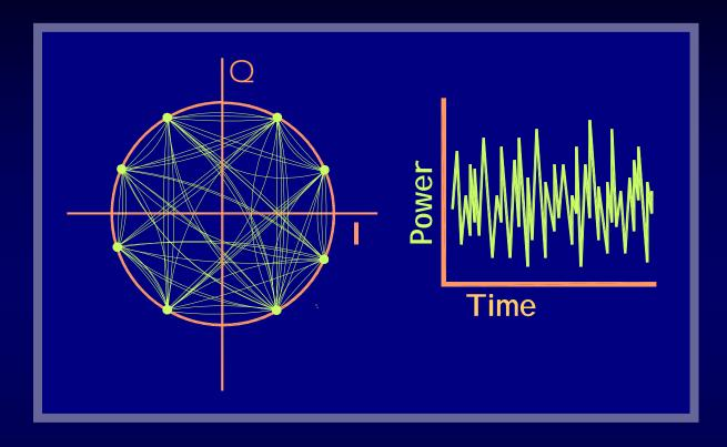
Transitions between the four quadrants cause psudorandom amplitude modulation
