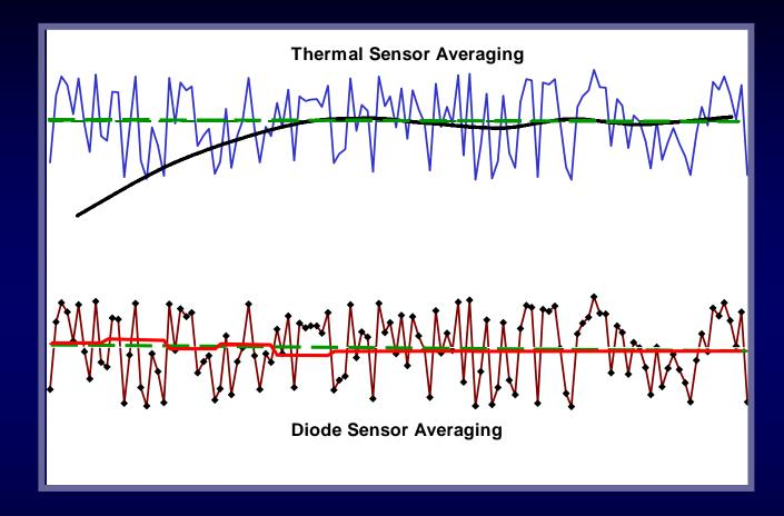
Multiple readings of normally distributed noise settles to average power
